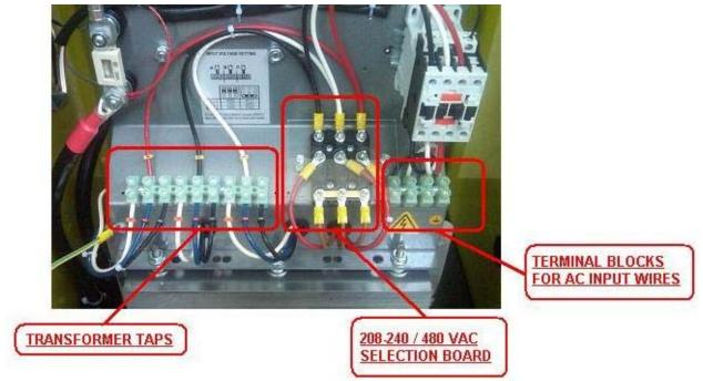
The charger must be connected to the AC input using an adequate cable and plug, with disconnect switch and fuses.
