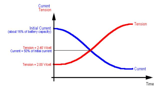
When the battery reaches the gassing voltage, the charge continues for one half of the time needed to reach the gassing voltage, with a minimum total time of 30 minutes.
